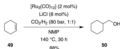
Scheme 18. Hydroformylation of cyclohexene ( 49 ) with CO 2 . [58]
